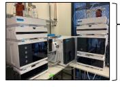
Targeted central carbon metabolism metabolites using a LC-Triple Quadrupole Mass Spectrometer (QqQ-MS).
